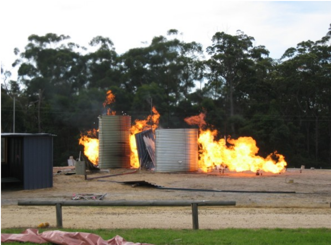
Figure C23 Tank three and five flame exposure.
