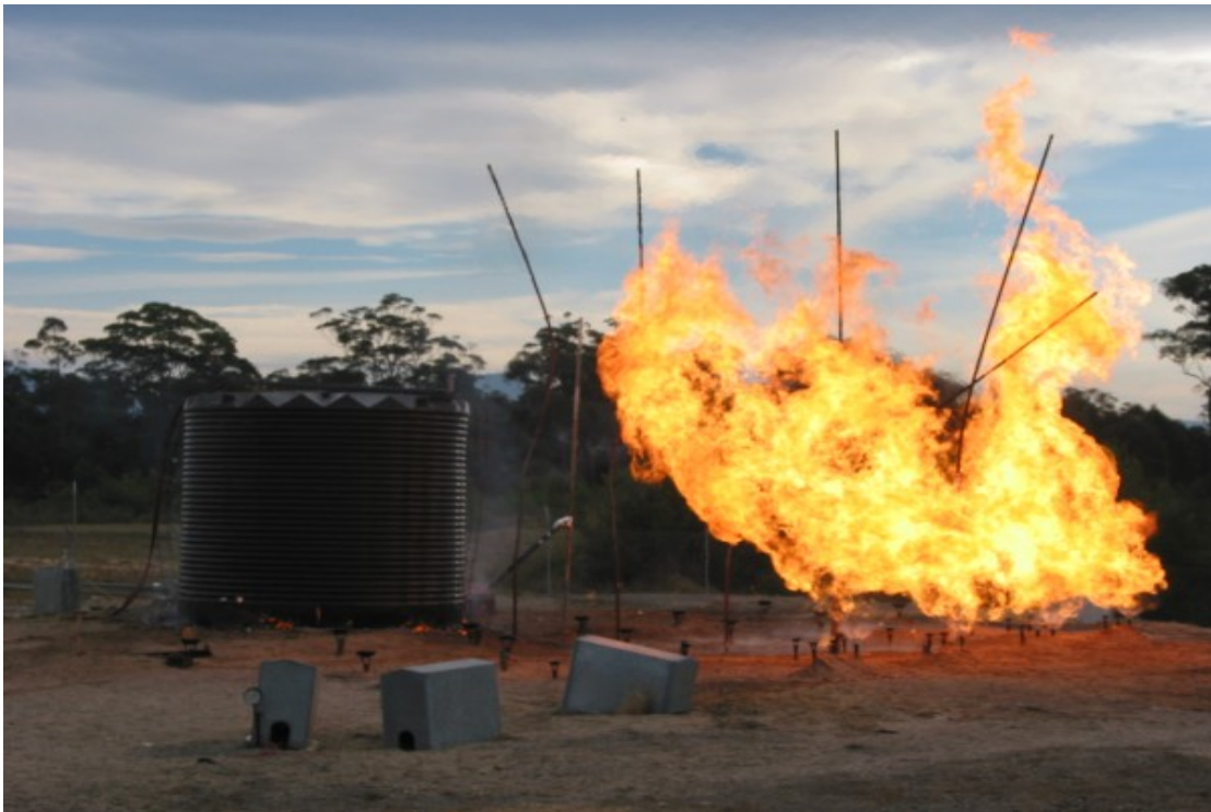
Figure C43 Tank 8 litter ignition and pre-radiation exposure.
