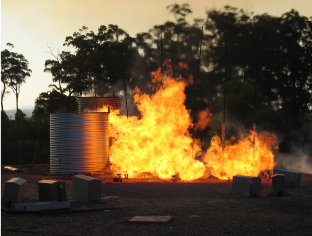
Figure C16 Tank three and five pre radiation flame contact.
