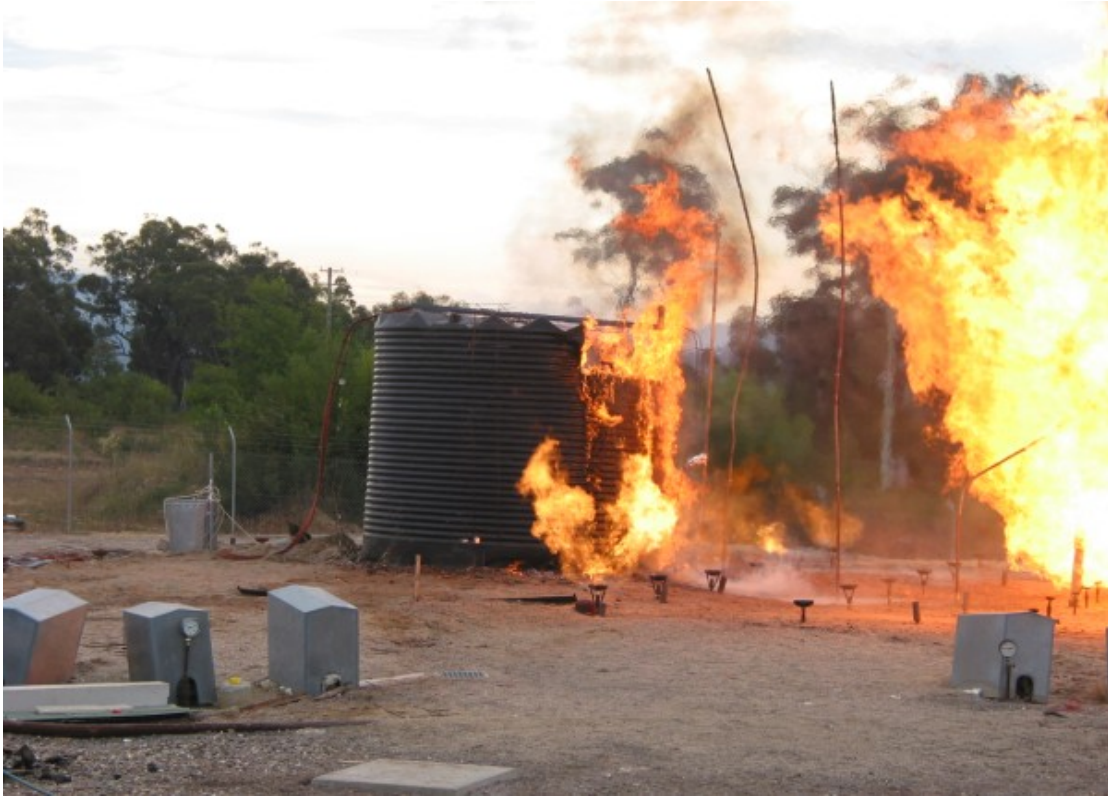
Figure C49 Tank 8 ignition as a result of litter ignition and pre-radiation and flame exposure.
