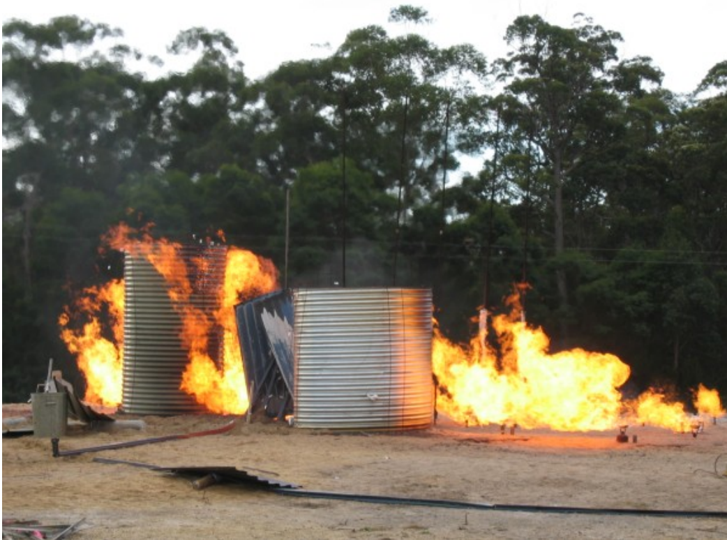
Figure C24 Tank three and five flame exposure.
