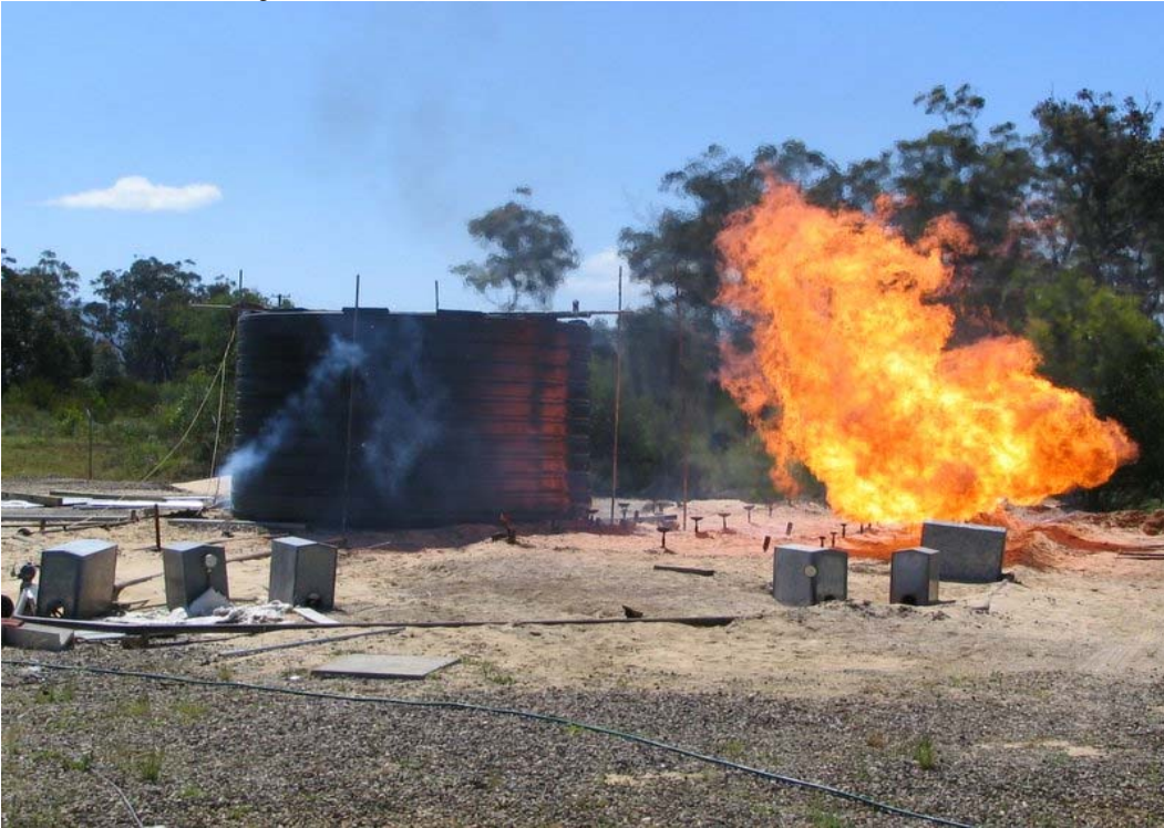
Figure C68 Tank 10 litter ignition and pre-radiation exposure.
