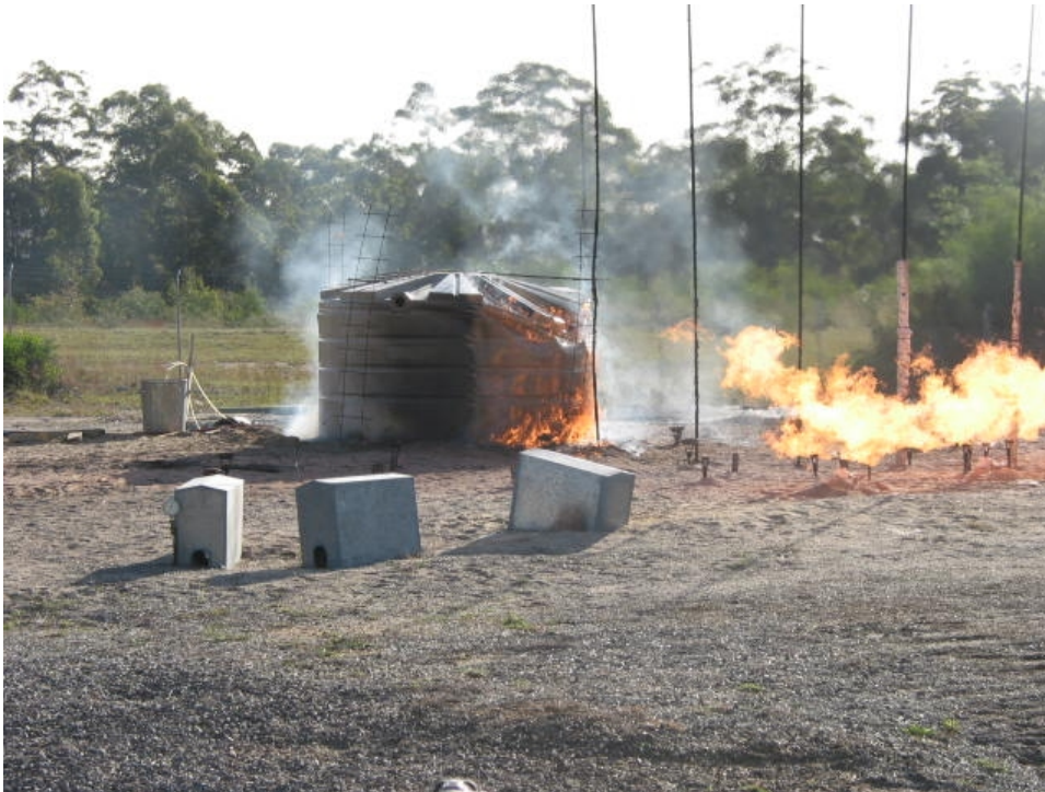
Figure 10 Experiment 5 - Pre-radiation exposure on polyethylene tank
