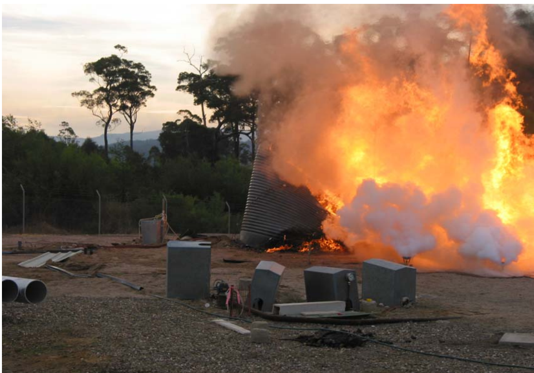
Figure C53 Tank 8 ignition and initial stages of failure due to structural fire exposure.
