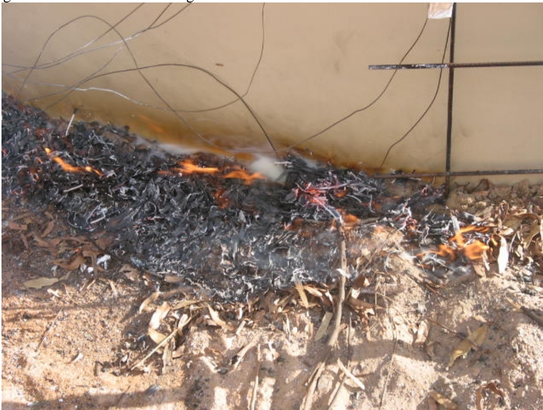
Figure C8 Tank six smouldering litter contacting exterior of tank.
