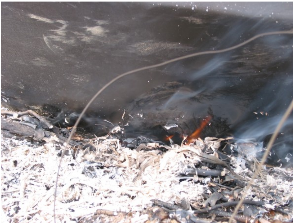
Figure 28 Experiment 18 - Leaf litter ignited exposure on polyethylene tank
