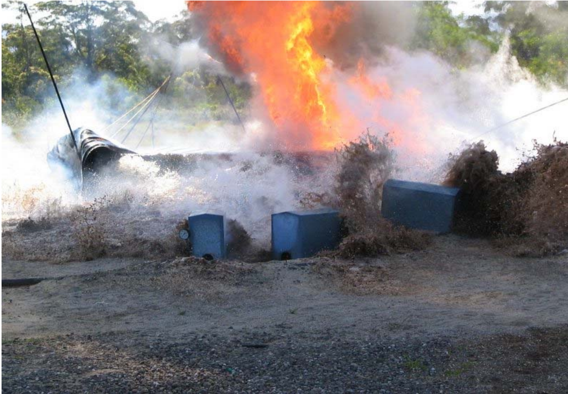
Figure C73 Tank 10 completely failing with contents flowing out due to flame exposure.
