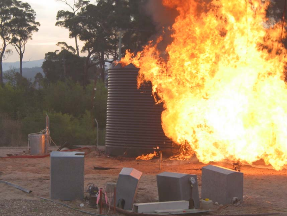
Figure C52 Tank 8 ignition due to structural fire exposure.
