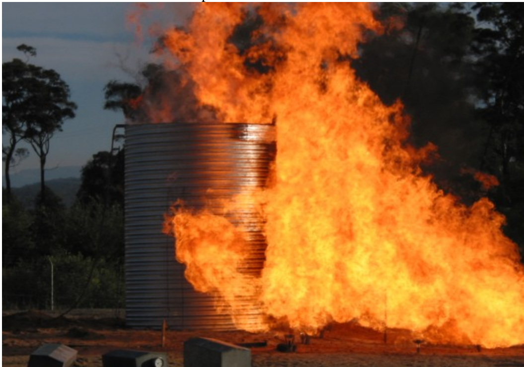
Figure C37 Tank 7 structural exposure.
