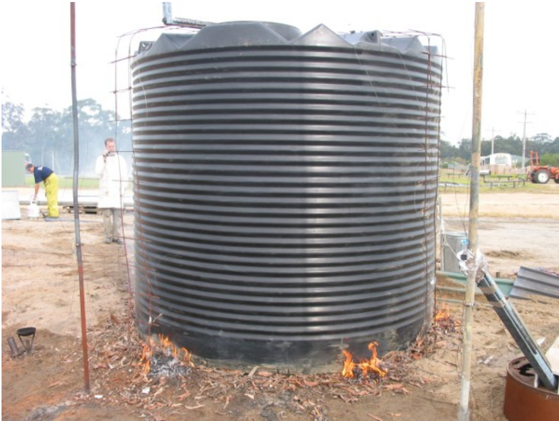
Figure C42 Tank 8 litter ignition .
