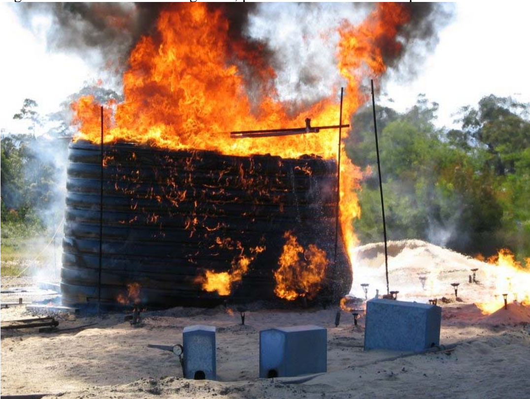
Figure C73 Tank 10 completely alight and about to fail as a result of litter ignition, pre-radiation and flame exposure.
