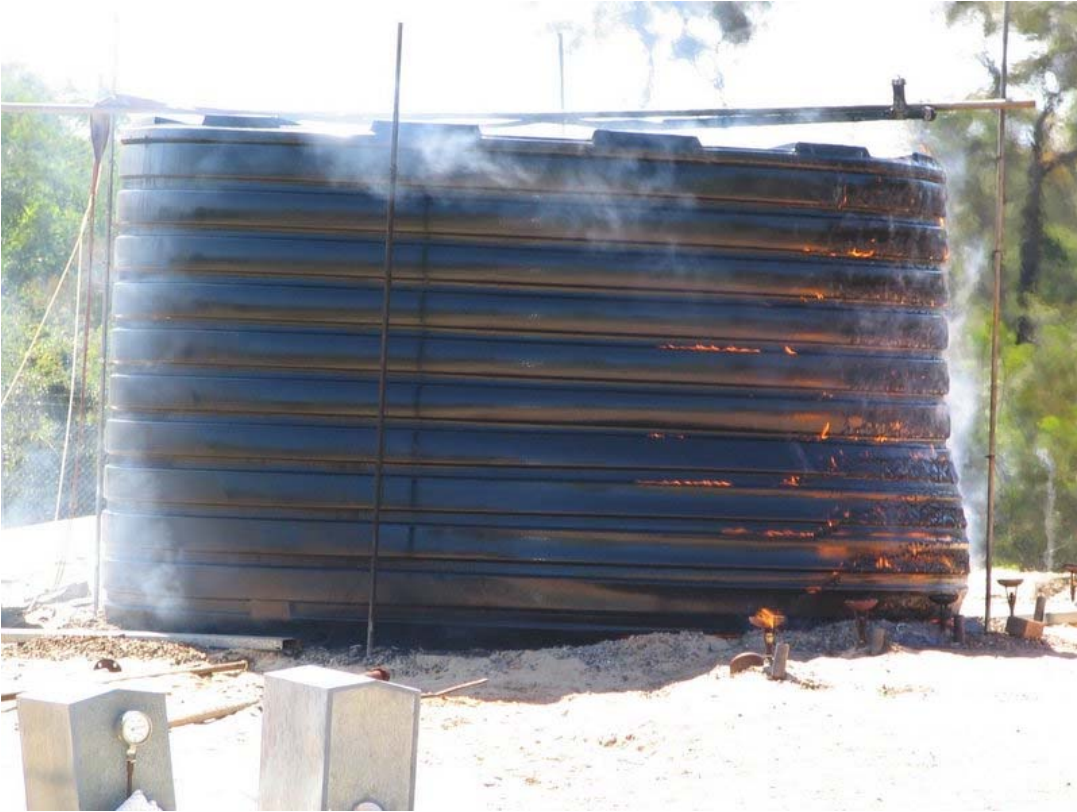
Figure C70 Tank 10 continuing to burn post the litter ignition and pre-radiation exposure.
