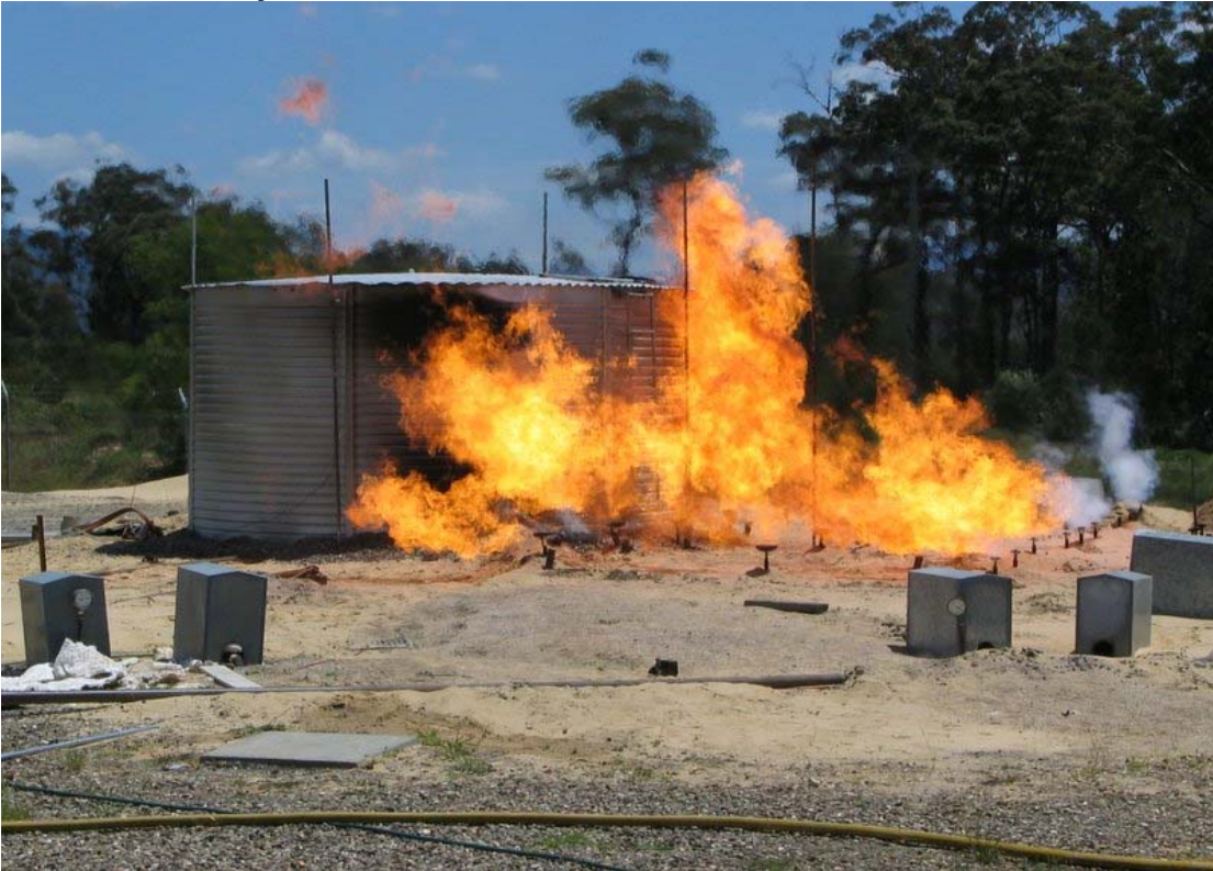
Figure C64 Tank 9, bladder tank structural exposure.
