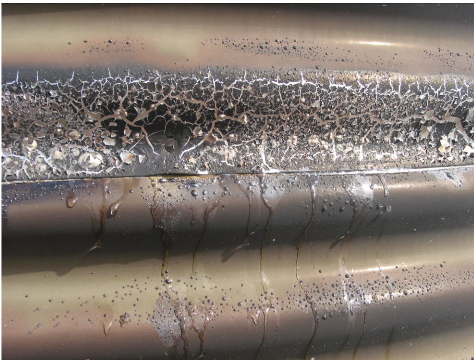
Figure 15 Experiment 9 - Leak from seams
