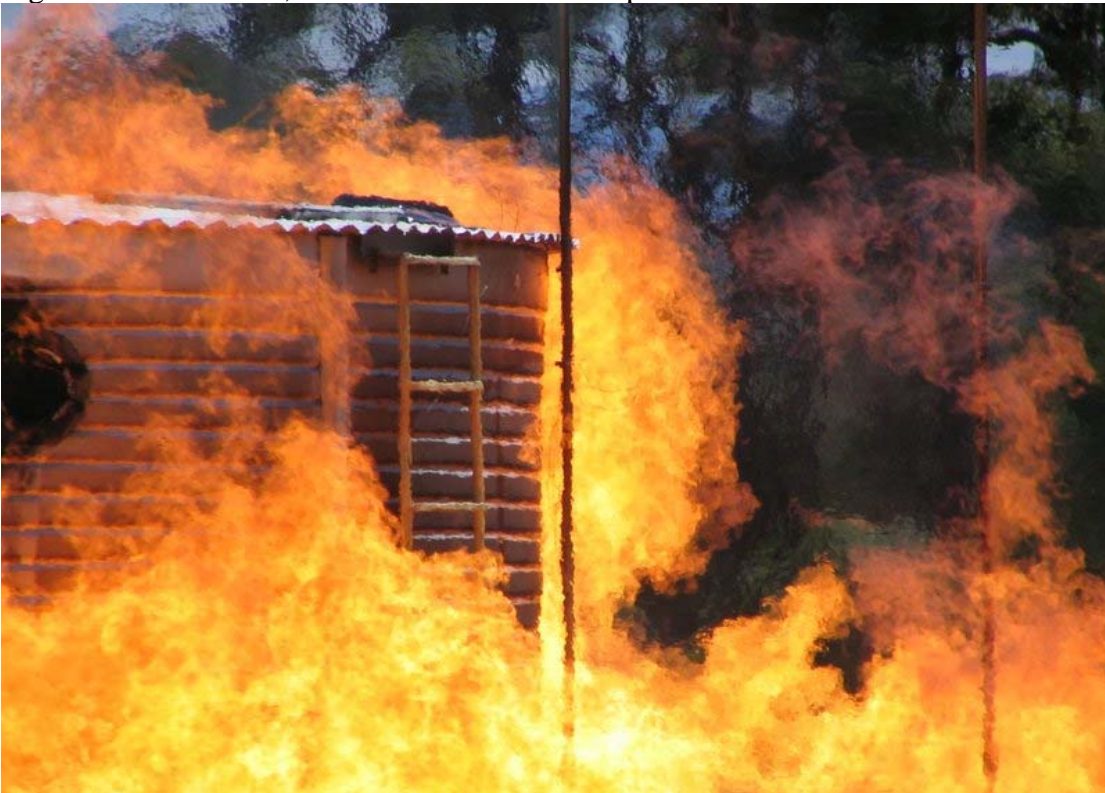
Figure C65 Tank 9, the bladder tank structural exposure.
