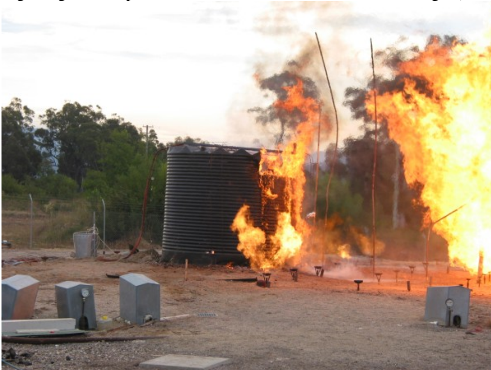
Figure 33 Experiment 20 - Polyethylene tank
