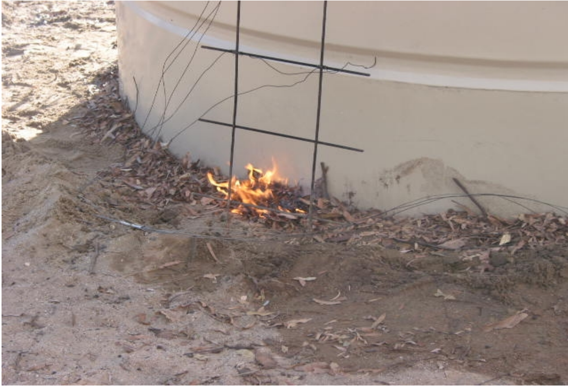
Figure C7 Tank six Litter ignition.
