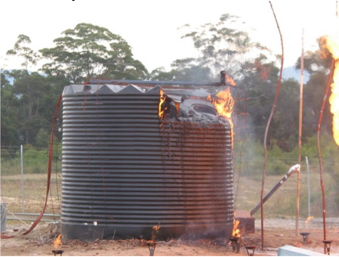
Figure C46 Tank 8 ignition as a result of litter ignition and pre-radiation and flame exposure.
