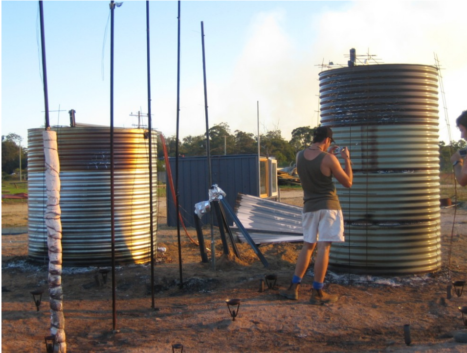
Figure 14 Experiment 9 - Pre-radiation and flame exposure on metal tank
