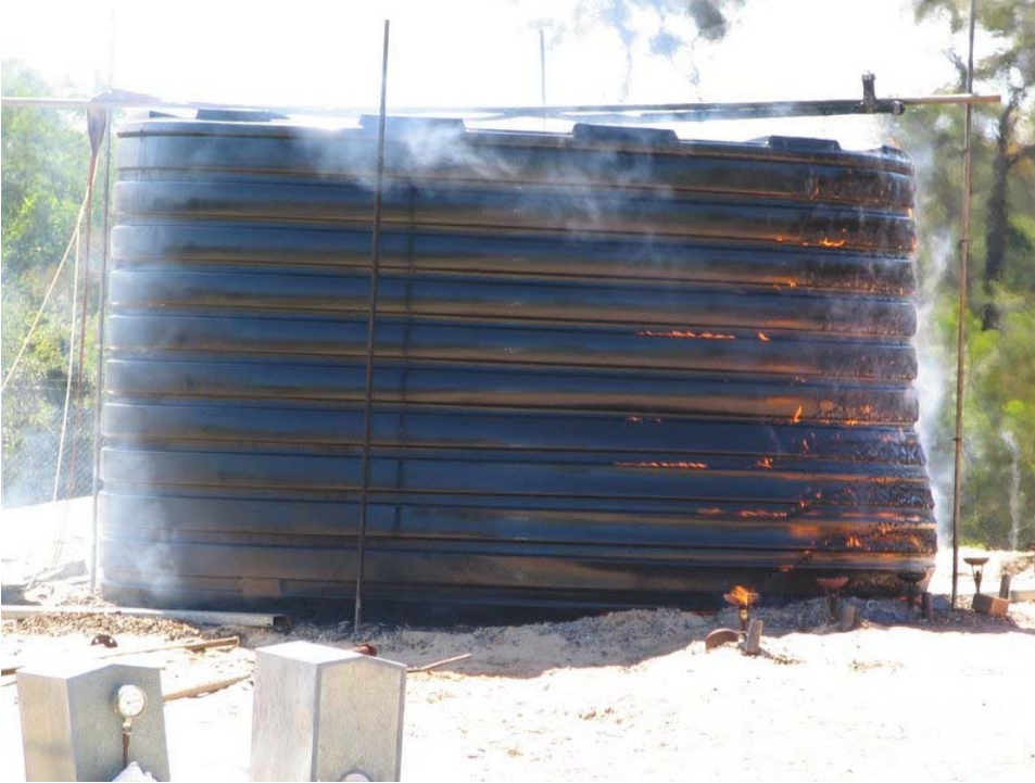
Figure 41 Experiment 25 - Leaf litter and pre-radiation exposure on used polyethylene tank
