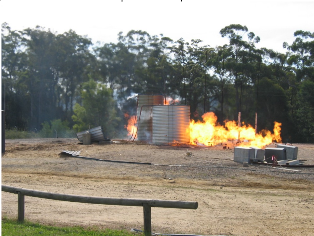
Figure C21 Tank three and five flame exposure.
