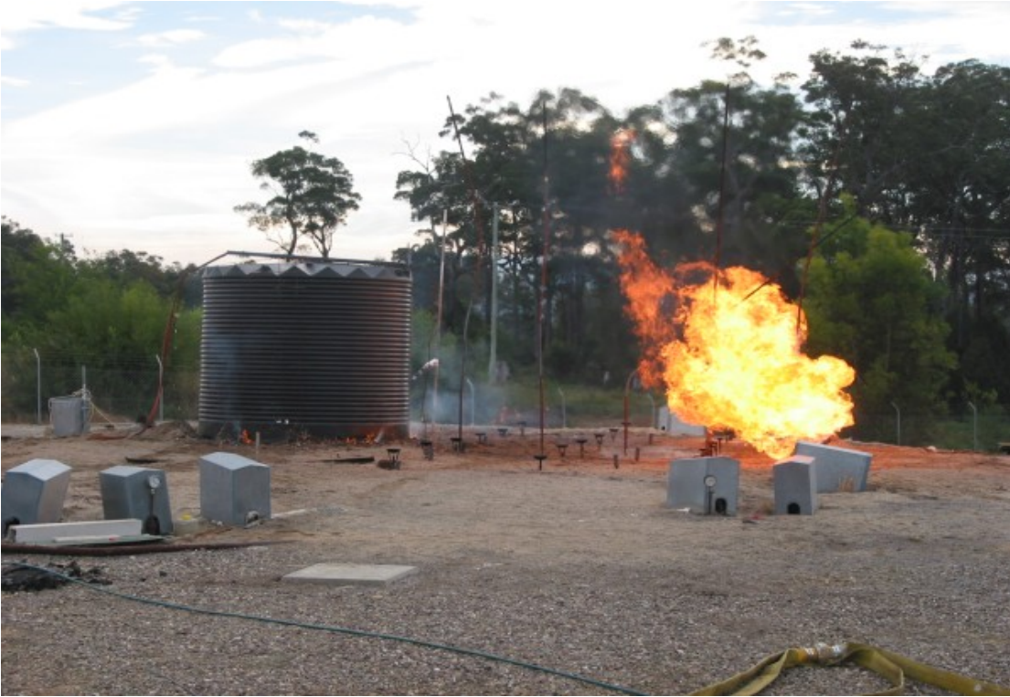
Figure C42 Tank 8 litter ignition and pre-radiation exposure.
