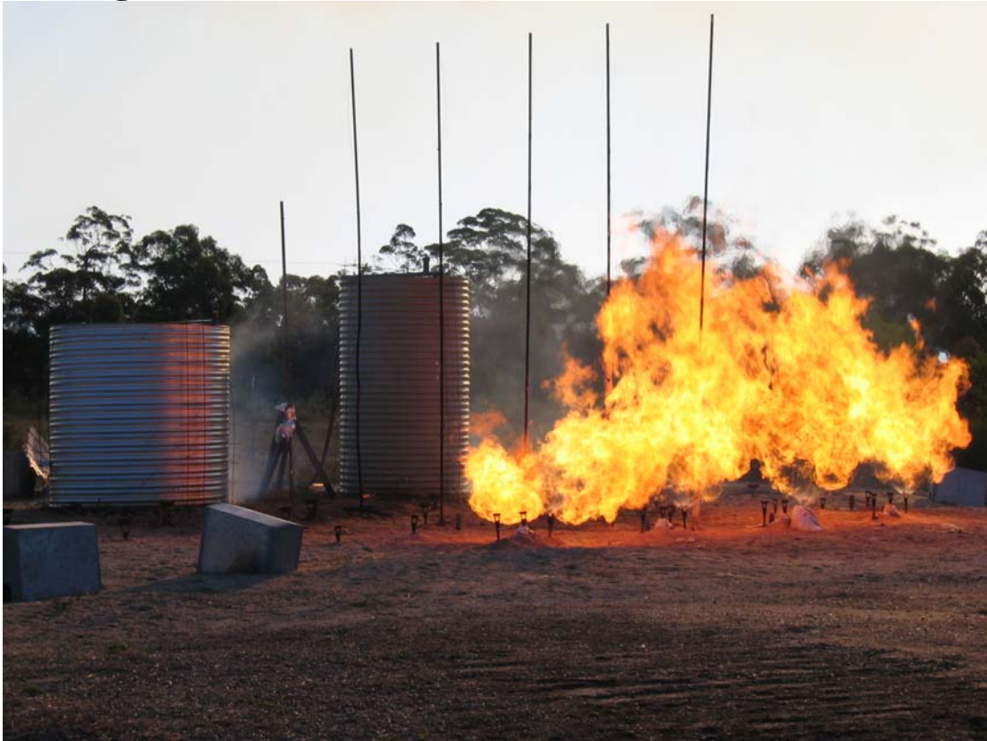
Figure C14 Tank three and five Pre Radiation exposure.
