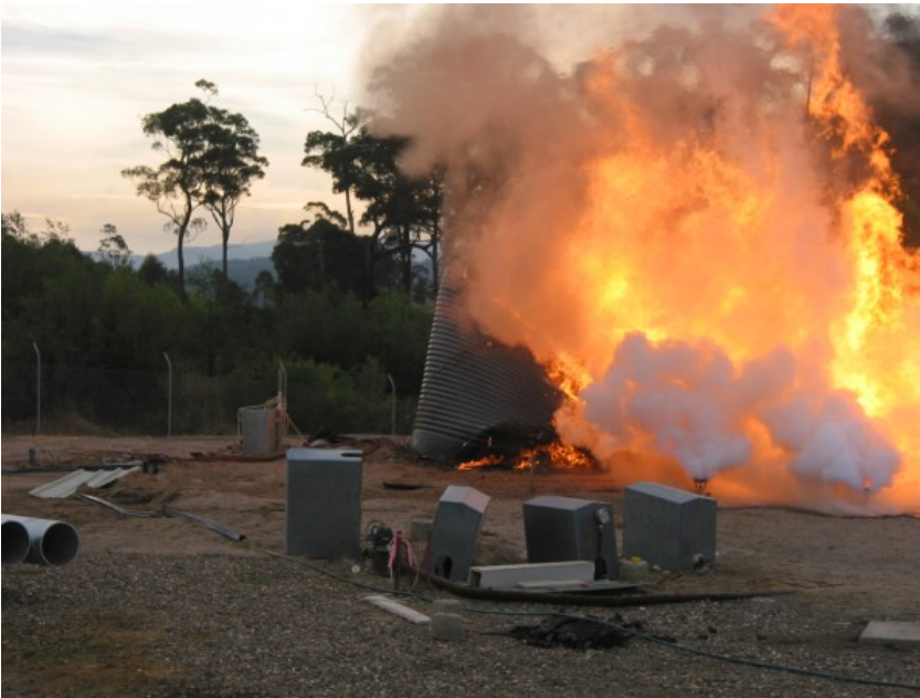
Figure 35 Experiment 21 polyethylene tank at two minutes into tests
