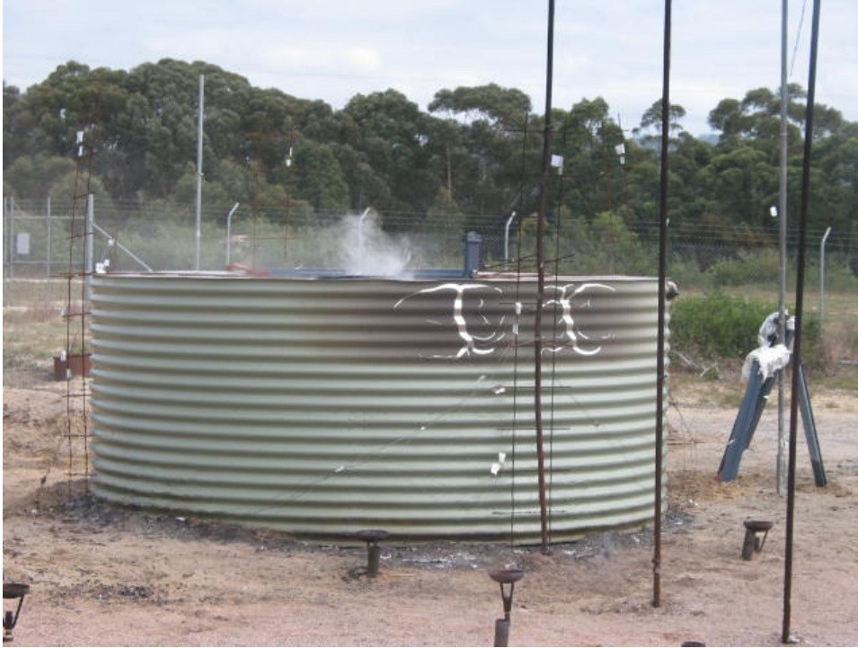
Figure 4 Experiment 1 - Leaf litter ignited and pre-radiation on metal coated water tank
