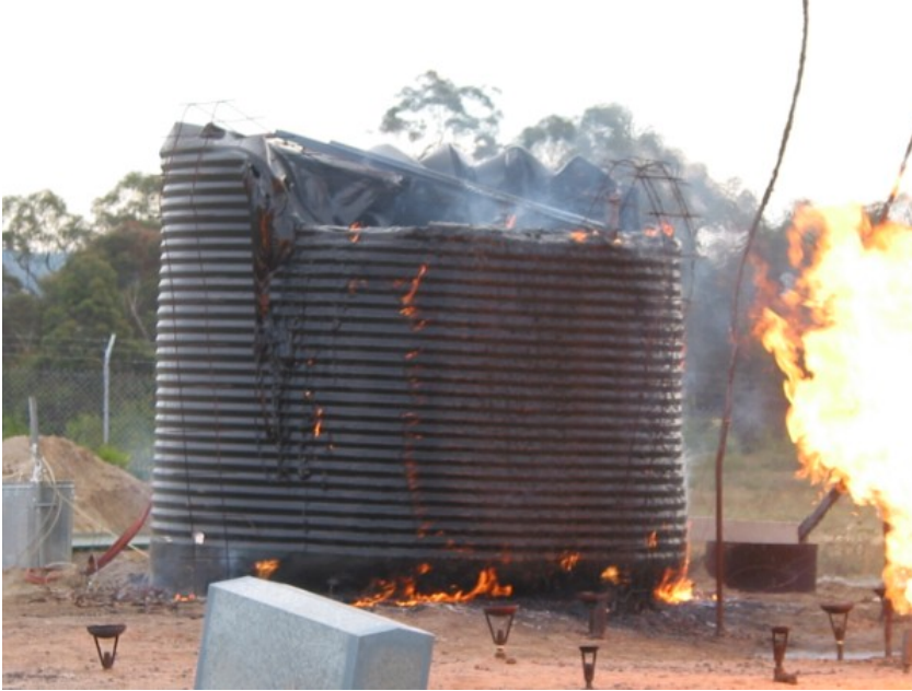
Figure 34 Experiment 20 – Pre-radiation and flame exposure on polyethylene tank
